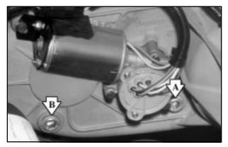
(A) Fill Plug (B) Drain Plug
